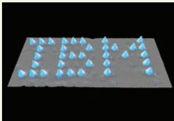
Figure 9 One way to repay a sponsor for supporting scientific research is to produce an image of their abbreviated name with xenon atoms on nickel and record it using scanning tunnel microscopy
