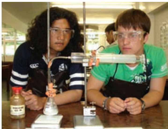
Figure 3 Roman Bulgakov from Russia and Tengku Omar Mokhtar from Malaysia, students at Atlantic College, using a gas syringe to follow the rate of reaction between calcium carbonate and hydrochloric acid
