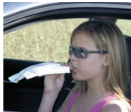
Figure 43 A potassium dichromate(VI) breathalyser being used in the early 1990s
