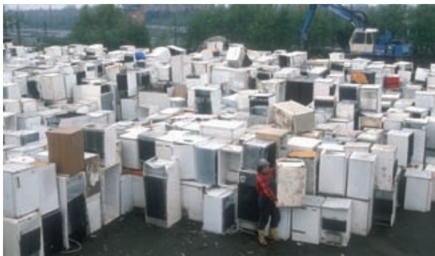
Figure 5 A pile of old refrigerators. Before old refrigerators can be broken up or recycled, the CFCs they contain must first be removed to prevent them from being released directly into the atmosphere.
