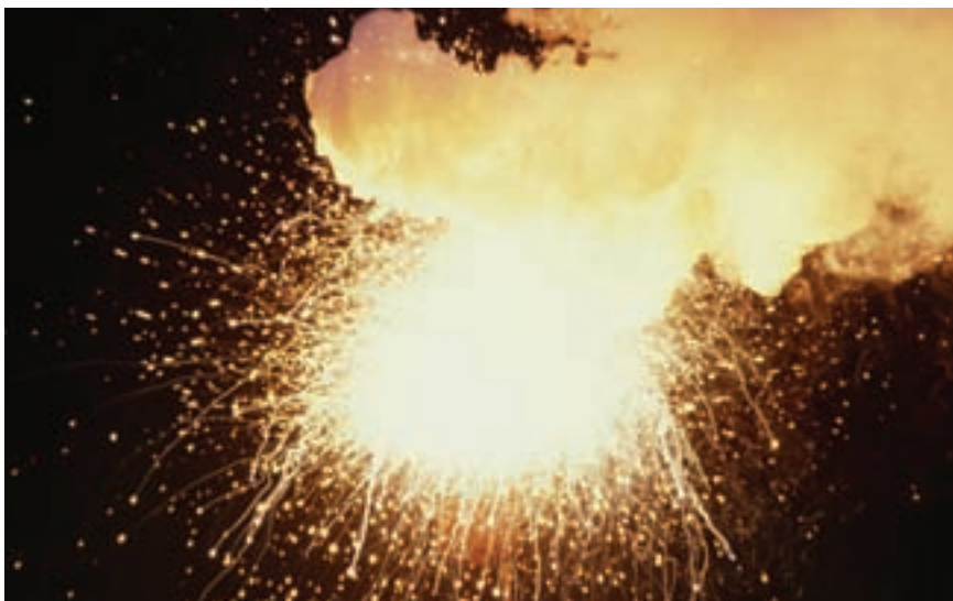
Figure 1 The "thermite reaction" is an example of an exothermic reaction. It is the reaction between a metal such as aluminium or magnesium with iron(III) oxide. The large amount of heat evolved can be used to weld sections of railway lines together.
