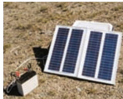
Figure 29 A solar powered battery charger
