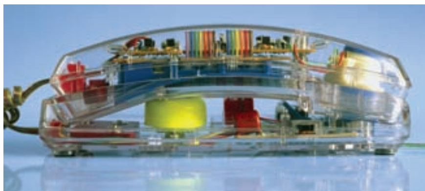
Figure 40 A telephone made with Perspex casing
