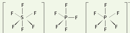
Figure 61 Bonding in sulfur hexafluoride, phosphorus pentafluoride and the hexafluorophosphorous ion, showing an “expanded octet”
