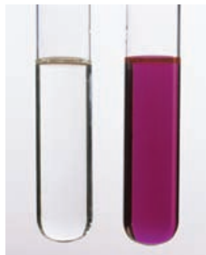
Figure 18 Two test tubes, one containing an acid and one containing an alkali. Both tubes contain phenolphthalein indicator. The acid forms a colourless solution and the alkali forms a pink solution.
