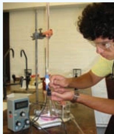
Figure 13 Jawad Al-Masannat from Jordan, a student from Atlantic College, using a pH meter during the acid-base titration
