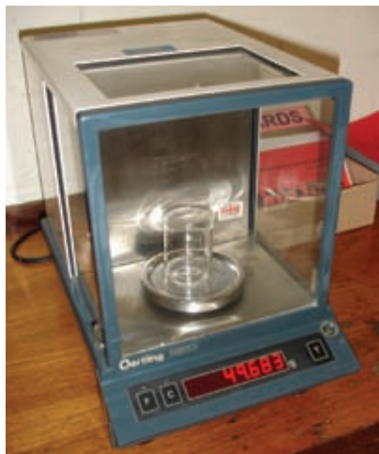
Figure 10 An analytical balance measuring to \pm 0.001 \text{ g}
