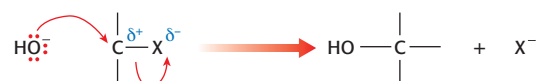
Figure 49 Nucleophilic substitution of halogenoalkanes with aqueous hydroxide ions, where X represents a chlorine, bromine or iodine atom. The carbon-to-fluorine bond is too strong for fluoroalkanes to undergo nucleophilic substitution.
