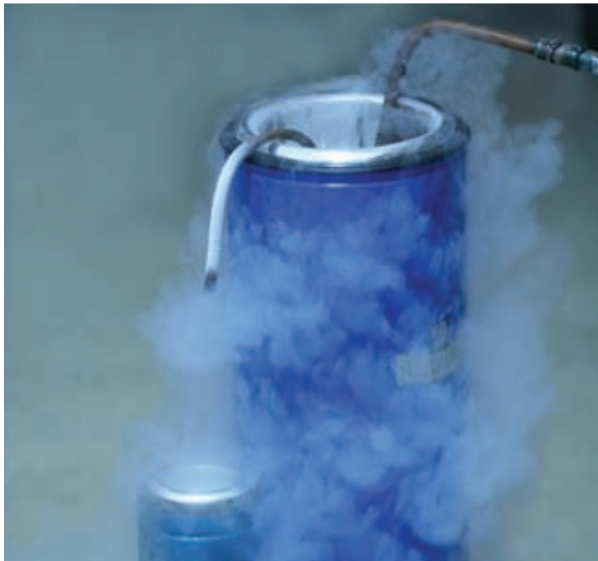
Figure 33 Liquid helium (boiling point -269\text{ }^{\circ}\text{C} ) being used to cool a spectrometer which needs to operate at very low temperatures
