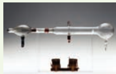
Figure 3 One of Thomson's original cathode ray tubes used to discover the electron
