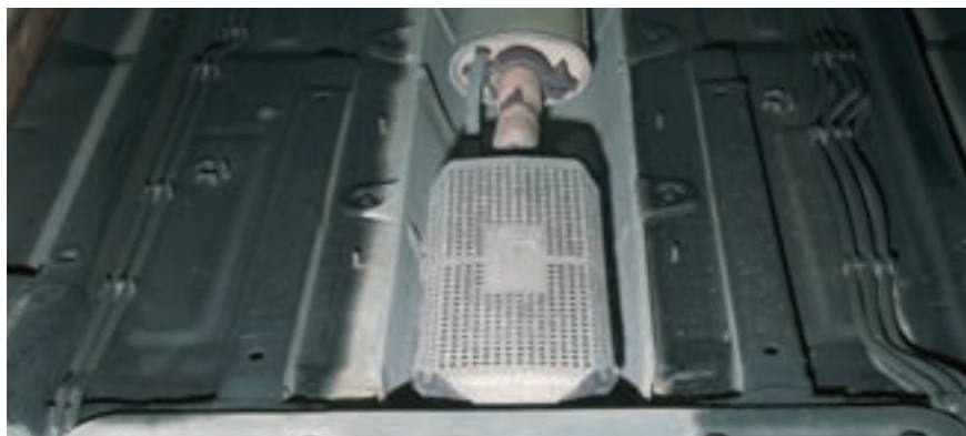
Figure 34 Precious metals adsorbed onto a mesh to increase their surface area for use as the heterogeneous catalyst in automobile catalytic converters
