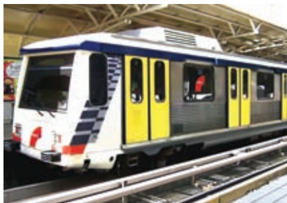
Figure 16 Using liquid crystals, the Light Rail Transit train in Singapore is able to fog out the windows when the train passes by residential flats, to protect the privacy of the flats’ occupants.
