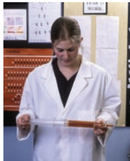
Figure 8 Sealed gas syringe containing nitrogen dioxide
