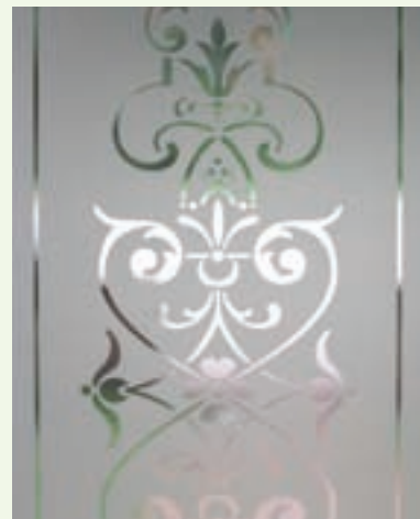
Figure 4 Hydrofluoric acid is a weak acid but is very corrosive and can be used to etch glass
