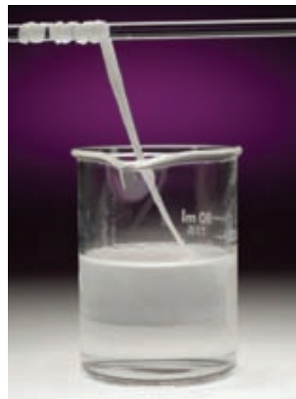
Figure 33 Making nylon - the nylon forms where the surface of the 1,6-diaminohexane solution meets the surface of the hexane-1,6-dioyl dichloride solution
