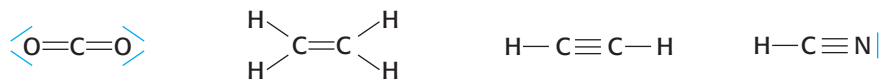
Figure 10 Lewis structures of carbon dioxide ( \text{CO}_2 ), ethene ( \text{C}_2\text{H}_4 ), ethyne ( \text{C}_2\text{H}_2 ) and hydrogen cyanide ( \text{HCN} )
