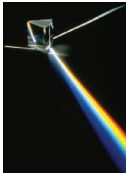
Figure 18 White light split into the different colours of the rainbow by a prism
