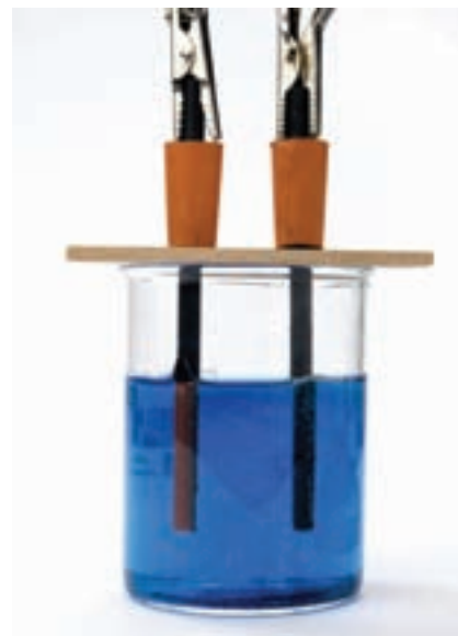
Figure 25 Copper sulfate solution being electrolysed with inert electrodes (Pt or graphite) to show oxygen coming off the positive electrode and copper being formed on the negative electrode
