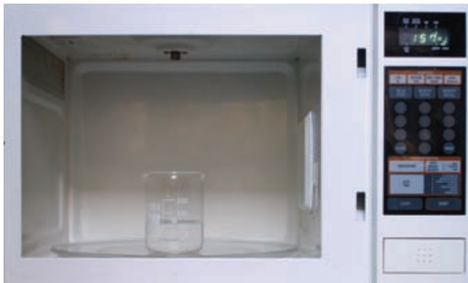
Figure 38 Microwave ovens work by heating polar water molecules due to their rapid rotation in an oscillating electric and magnetic field
