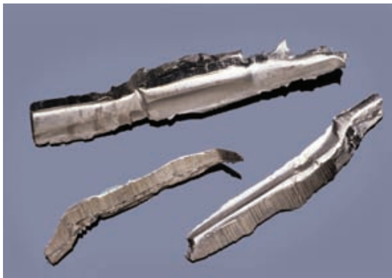
Figure 10 Pieces of solid nickel. In their finely divided form they are used as a heterogeneous catalyst to hydrogenate alkenes.
