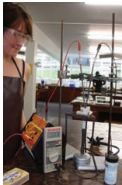
Figure 18 Rebecca Pedrick-Case an IB student from Wales, UK, showing that lead bromide conducts an electric current when molten
