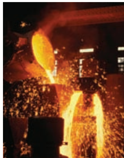
Figure 4 Steel being poured from an oxygen converter
