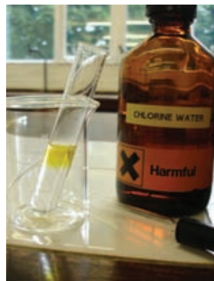
Figure 20 Chlorine water reacting with a solution of potassium bromide to produce bromine
