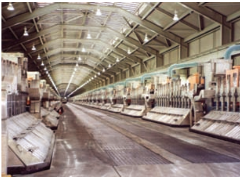
Figure 6 Rows of electrolytic cells in an aluminium plant in Bahrain
